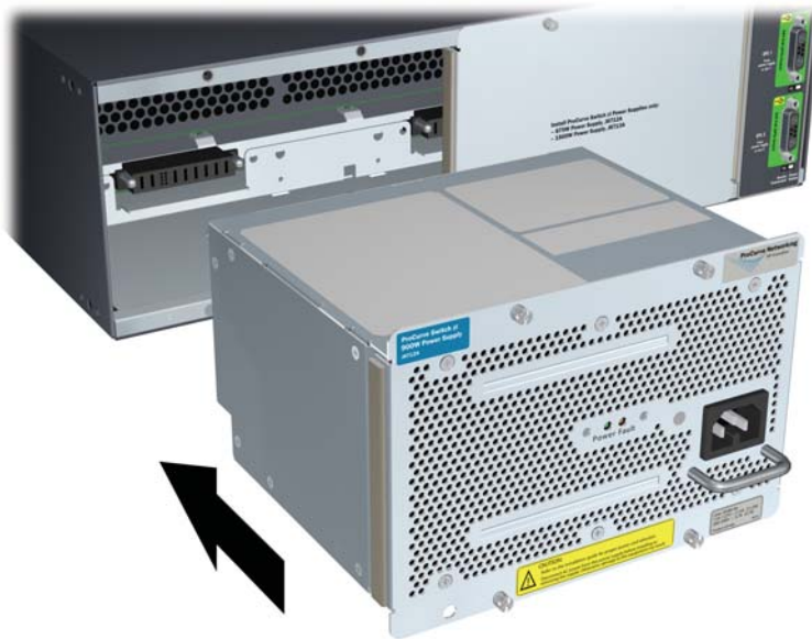
Figure 2-5. Installing a power supply
